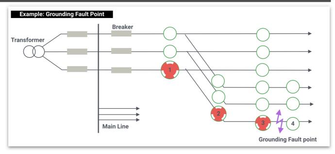
Note: The diagram above indicate that the fault section is between the point 3 and point 4.
